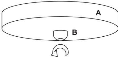
1. Carefully unpack parts. Remove the Canopy (A) from the Mounting Plate by unscrewing the Retainer (B). Fully remove the Retainer from the threaded nipple, then pull the canopy from the Mounting Plate.
