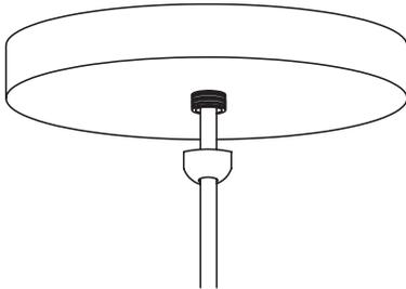
6. Lift the canopy up to the ceiling and tighten with the Retainer, but do not overtighten.
