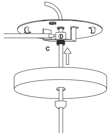
**CAUTION:** Overtightening the set screw could pierce cord and prevent pendant from operating.
