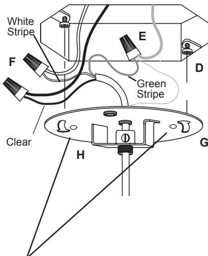
3. Install the provided Mounting Screws (D) into the Outlet Box, leaving 1/4" of threading as shown.
