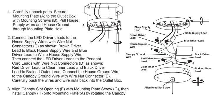
Clock-wise. Then tighten the Mounting Plate Screws (G) to secure Canopy in place.
