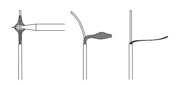
Once the inner conductor is exposed, it can now be separated from the braiding. Slide the pointed object between the inner conductor and the braiding, as shown. Gently wedge the inner conductor apart from the braiding. Now twist the braiding tightly into a conductor.
