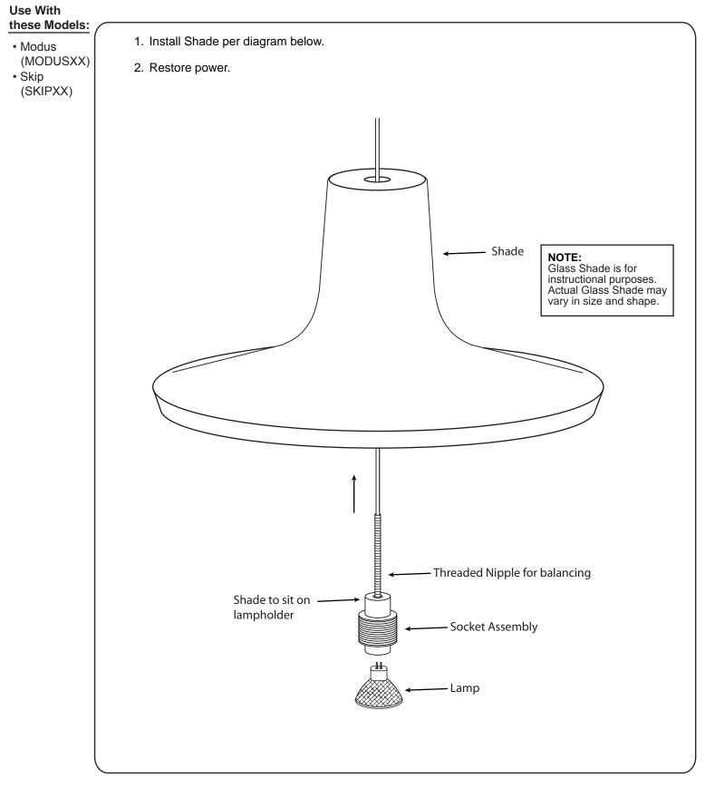
All electrical connections and the installation of this fixture must be in agreement with local codes, ordinances or the NEC (National Electric Code) or CEC (Canadian Electrical Code). Do not connect this fixture to an electrical system that does not provide a means for equipment grounding.
