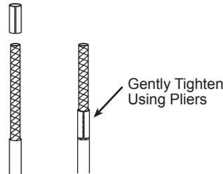
4. Remove the exposed braiding by pulling away from the center conductor, then cutting off excess. Leave 1/16" of braided material or less.
