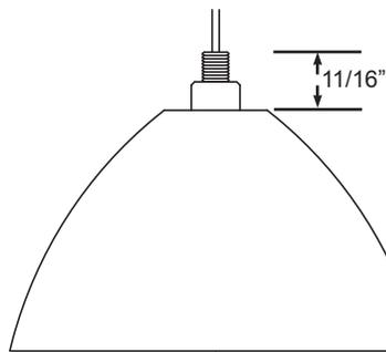
This Pendant Cord Set has been designed to allow the Glass Shade to either rest freely or to be locked in position. To lock down Glass Shade, adjust the Threaded Nipple as shown. Otherwise, thread completely into Lampholder.
