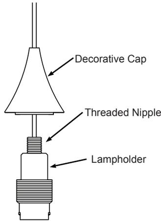
Prior to installing Quick Connect Fitting, the Decorative Cap and Threaded Nipple must be installed. The Decorative Cap and Threaded Nipple do not need to be secured at this time.
