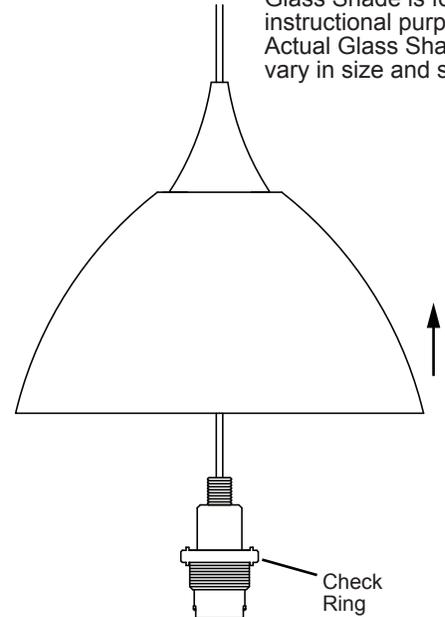
Install the Glass Shade by positioning up over the Lampholder and thread on the Check Ring completely, as shown.
