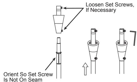
9. Insert the post of the Quick Connect Jack into the Quick Connect Adapter. Thread the top half of the conical section until it seats with the adapter.
