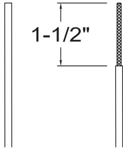
Carefully measure the desired length of cord and cut off the excess. It is important to leave an additional 6" that will be inside the canopy for connection to your transformer. Using the 10 AWG setting, strip off 1-1/2" of outer teflon jacket with a pair of wire strippers.
