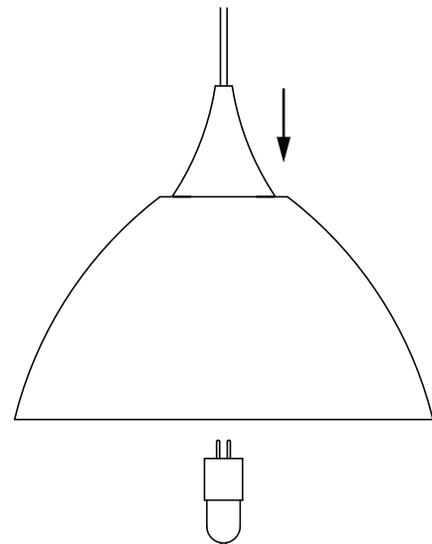
Relamp with a low-pressure type lamp, either xenon or halogen. Packaging of this lamp will typically indicate that it's "Suitable For Use in an Open Fixture" or marked with the symbol shown.
