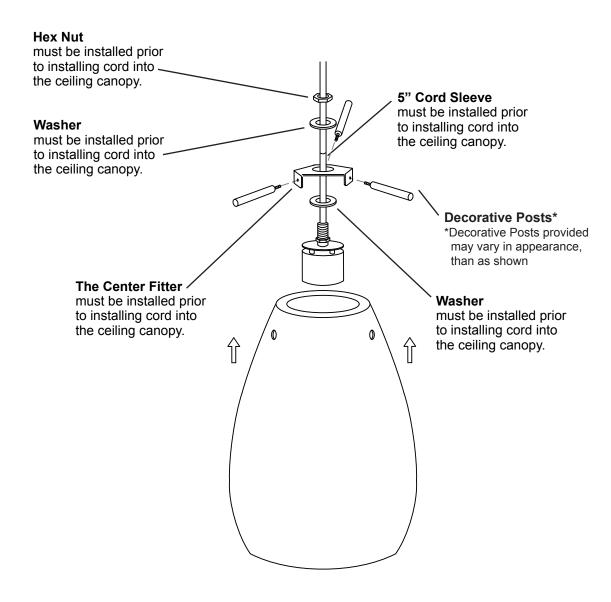
All electrical connections and the installation of this fixture must be in agreement with local codes, ordinances or the NEC (National Electric Code) or CEC (Canadian Electrical Code).
