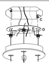
2. Install the provided Mounting Screws (C) into the Outlet Box, leaving 1/4" of threading as shown. Pull the House Wires from the Outlet Box and extend through the center opening in the Mounting Plate (D).
