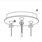
1. Carefully unpack parts. Remove the Canopy (A) from the Mounting Plate by unscrewing the three (3) Retainers. Fully remove the Retainers from the threaded nipple, then pull the canopy from the Mounting Plate.
