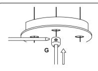
4. Prior to installing the canopy, the cord length must be adjusted.
