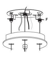
3. Shorten the three (3) cables to the desired length by pushing the cable up through the Cable Retainers (F). Trim off the excess cable length, leaving about 3" of slack for final adjustment.
