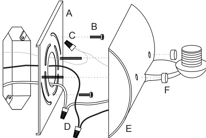
1. Carefully unpack parts. Remove Cap Nuts (F) to release Mounting Plate from Canopy.
