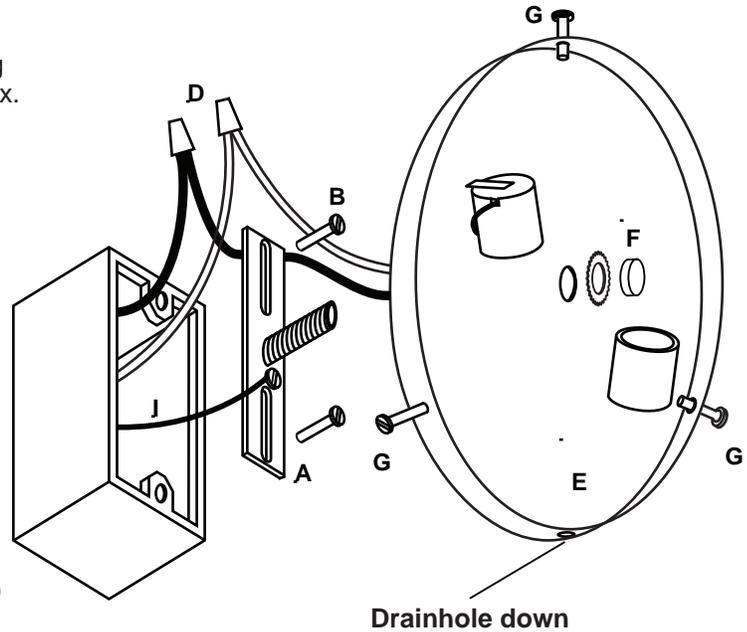
7. Partially install the retaining screws (G) into the canopy. The number of retaining screws will vary dependant upon the fixture model.
