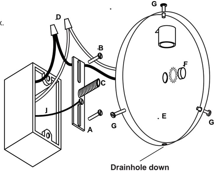
7. Partially install the retaining screws (G) into the canopy. The number of retaining screws will vary dependant upon the fixture model.
