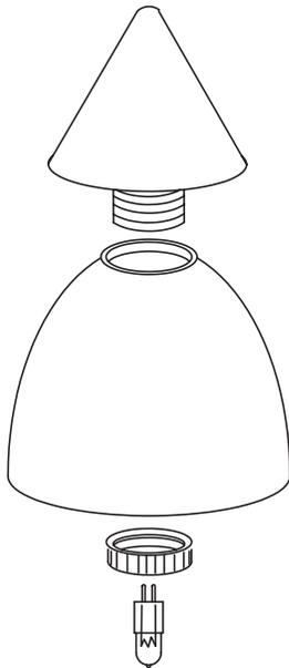
6. To attach the glass, you must first remove the Threaded Checking from the socket. Place the glass shade over the socket and secure with the Threaded Checking.
