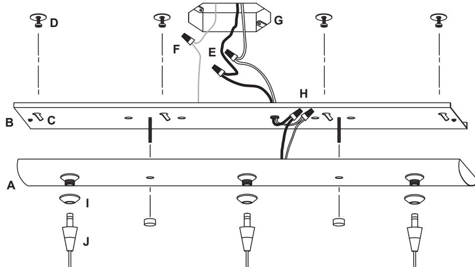
**This fixture has the electrical leads positioned for a center feed, with 10" offset capability.**
