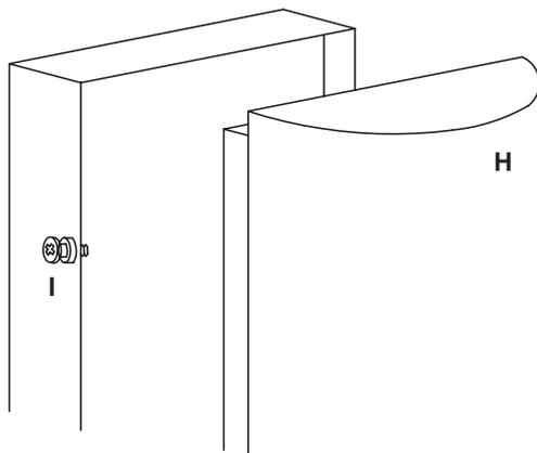
7. Gently position Glass Diffuser (H) into the Backplate. Secure with the four retaining screws (I).
