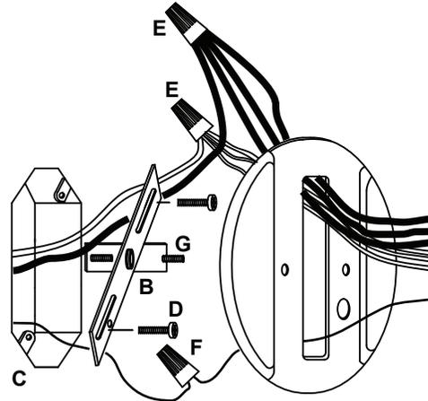
5. Align the circular openings on the Backplate and Canopy with the Threaded Posts (G) on the Mounting Plate. Push the Canopy and Backplate over the Threaded Posts until the Canopy is flush with the wall, then secure with the Cap Nuts.
