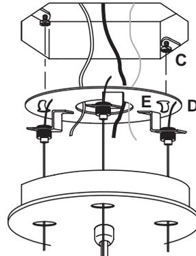
2. Install the provided Mounting Screws (C) into the Outlet Box, leaving 1/4" of threading as shown. Pull the House Wires from the Outlet Box and extend through the center opening in the Mounting Plate (D).
