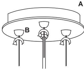
1. Carefully unpack parts. Remove the Canopy (A) from the Mounting Plate by unscrewing the three (3) Retainers. Fully remove the Retainers from the threaded nipple, then pull the canopy from the Mounting Plate.
