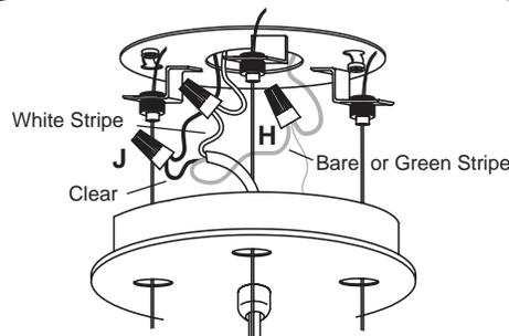
5. Attach the the bare copper fixture ground wire and bare (or green striped) ground conductor from the cord to the supply ground and secure with provided Wire Nut Connector (H). Connect the cord conductors from the fixture cord to the supply conductors with Wire Nut Connectors (J) as shown: Cord conductor with white stripe to white supply wire and clear cord conductor to black supply wire.
