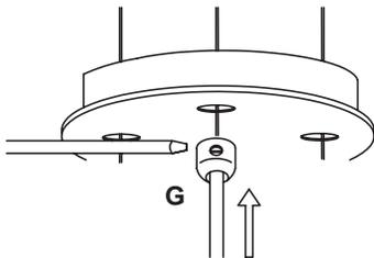
4. Prior to installing the canopy, the cord length must be adjusted. Loosen the set screw on the Strain Relief (G), the feed the cord up through until reaching the desired length. Tighten the set screw until the cord is firmly in place.
