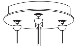
6. Prior to replacing the canopy, push the house wiring and wrenuts up through the center opening and into the Outlet Box.
