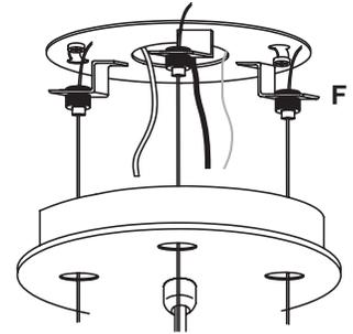
3. Shorten the three (3) cables to the desired length by pushing the cable up through the Cable Retainers (F). Trim off the excess cable length, leaving about 3" of slack for final adjustment.
