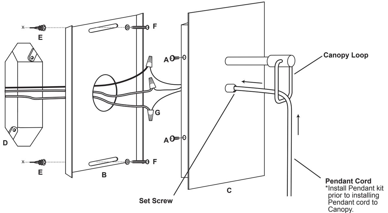
1. Carefully unpack parts. Loosen Canopy Screws (A) to release the Mounting Plate (B) from Canopy (C).
