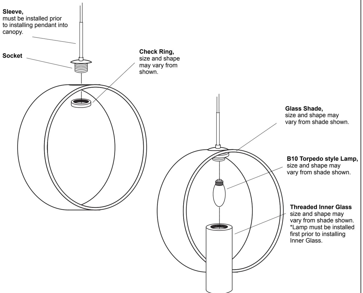
All electrical connections and the installation of this fixture must be in agreement with local codes, ordinances or the NEC (National Electric Code) or CEC (Canadian Electrical Code).
