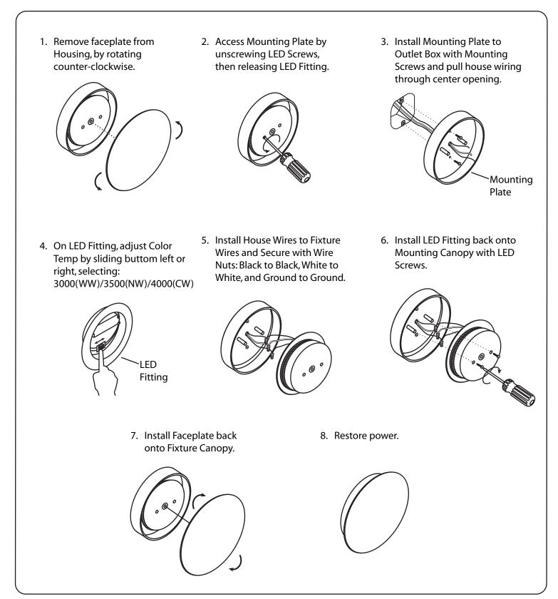
All electrical connections and the installation of this fixture must be in agreement with local codes, ordinances or the NEC (National Electric Code) or CEC (Canadian Electrical Code). Do not connect this fixture to an electrical system that does not provide a means for equipment grounding.
