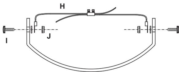
7. Remove Cable Kit from bag, then release Cable Assembly (H) by removing the Decorative Fastener (I).
