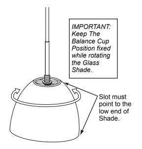
B. With the Knurled Nut secured down, rotate the Glass Shade so that the slot of the Balance Cup points to the lowest end of the Glass Shade.
