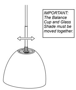
C. Slide both the Glass Shade and the Socket Assembly into a new position along the slot in the Balance Cup that will level the Glass Shade. It may be necessary to loosen the Knurled Nut during this step.
