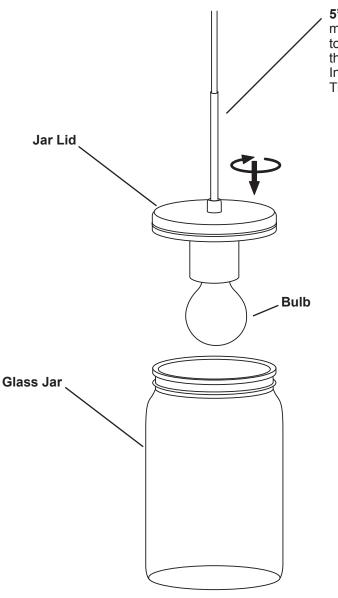
5" Cord Sleeve must be installed prior to installing cord into the ceiling canopy. Insert end firmly into Threaded Socket Holder.
