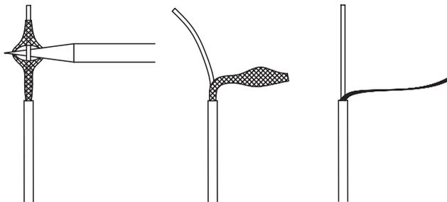
Once the inner conductor is exposed, it can now be separated from the braiding. Slide the pointed object between the inner conductor and the braiding, as shown. Gently wedge the inner conductor apart from the braiding. Now twist the braiding tightly into a conductor.
