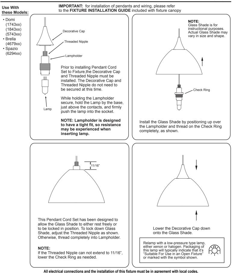
ordinances or the NEC (National Electric Code) or CEC (Canadian Electrical Code). Do not connect this fixture to an electrical system that does not provide a means for equipment grounding.
