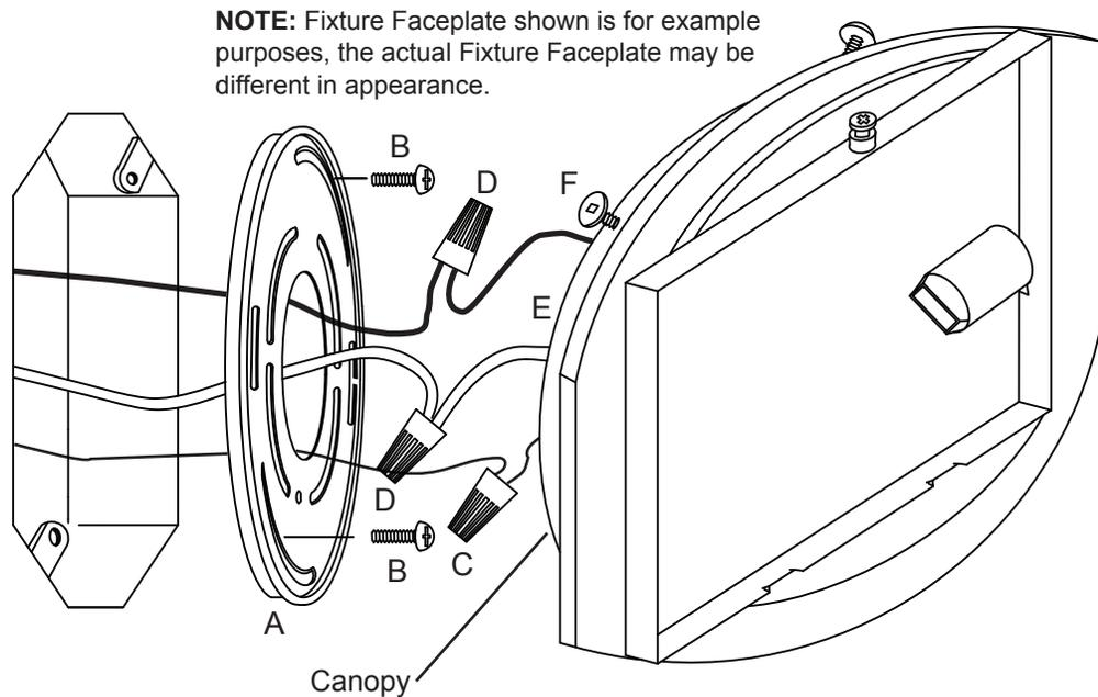
1. Carefully unpack parts. Loosen the three (3) Allen Head Screws (F) to release the Mounting Plate (A) from Canopy (E) using the Allen Wrench provided.
