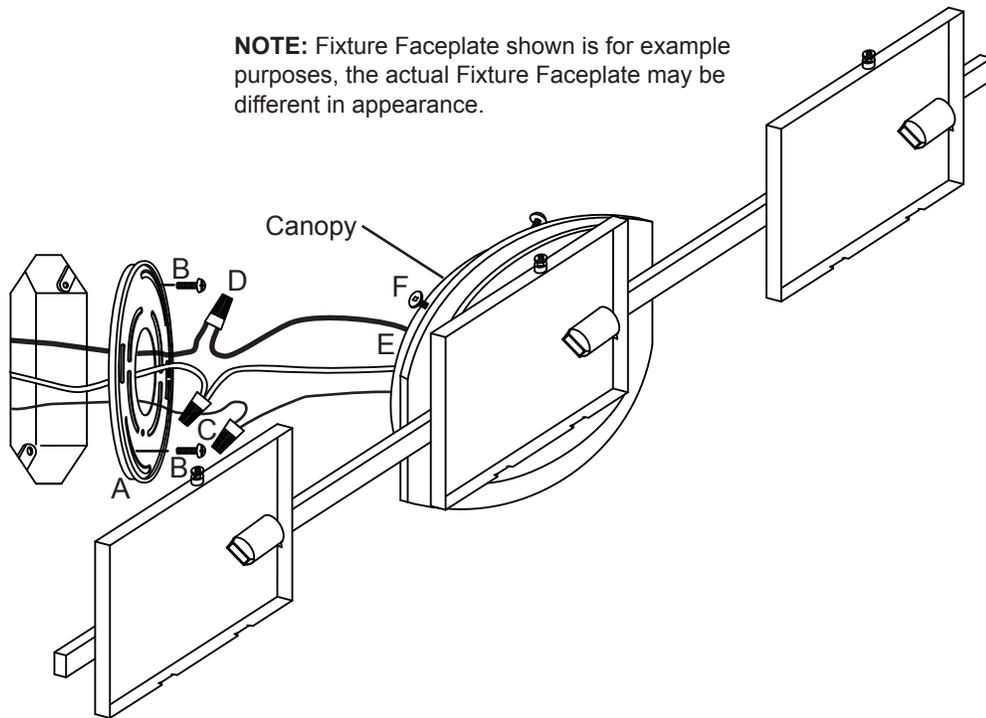
1. Carefully unpack parts. Loosen the three (3) Allen Head Screws (F) to release the Mounting Plate (A) from Canopy (E) using the Allen Wrench provided.
