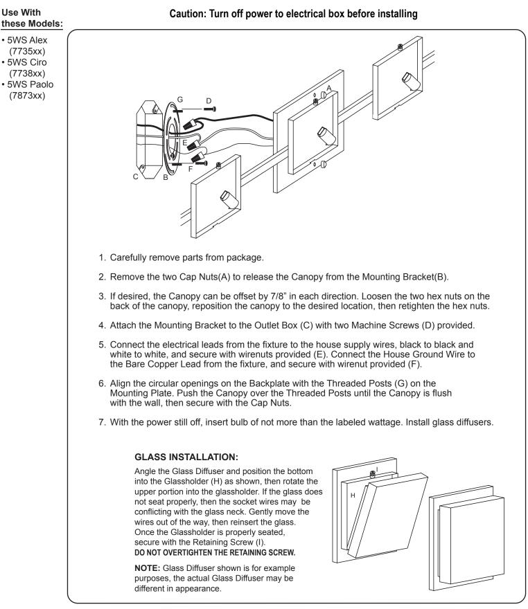
All electrical connections and the installation of this fixture must be in agreement with local codes. ordinances or the NEC (National Electric Code) or CEC (Canadian Electrical Code). Do not connect this fixture to an electrical system that does not provide a means for equipment grounding.
