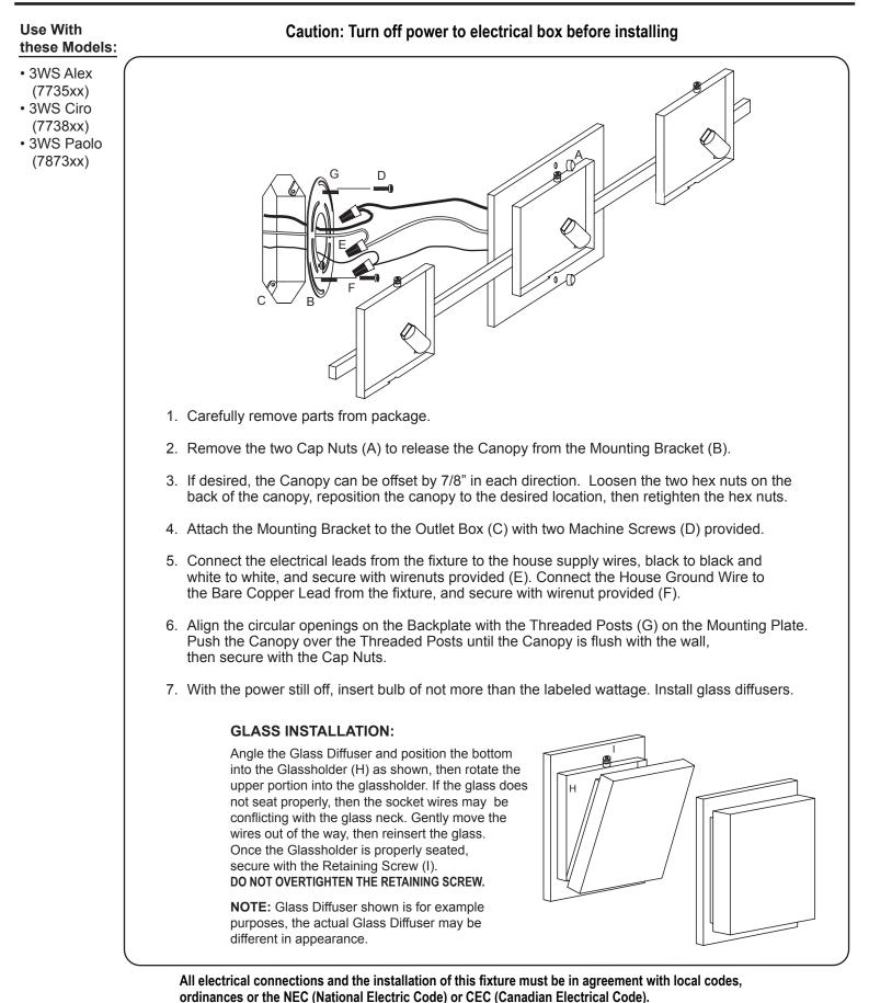
Do not connect this fixture to an electrical system that does not provide a means for equipment grounding.
